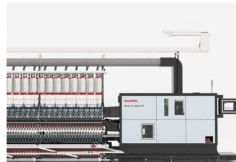
Zinser 51 with compacting unit Zpact FX © 2026 Saurer
