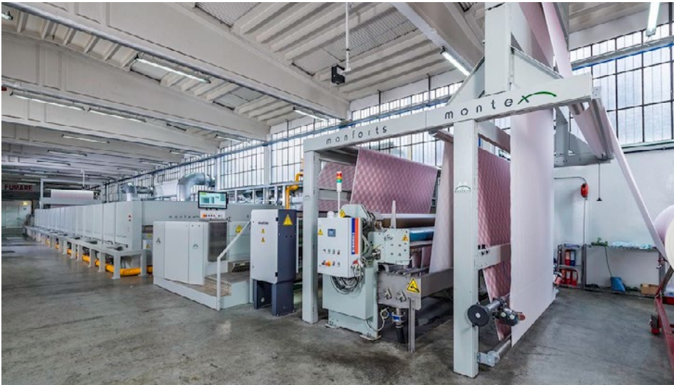
Monforts Montex stenters are still the industry standard for the fabric finishing industry © 2026 Monforts
