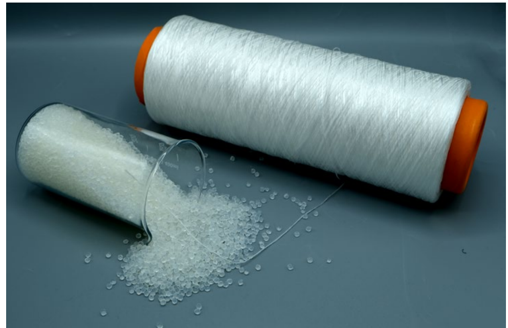
Fig. 1: A spool of filament yarn spun at the ITA from bio-based polyamide (Source & Copyright ©: ITA)
